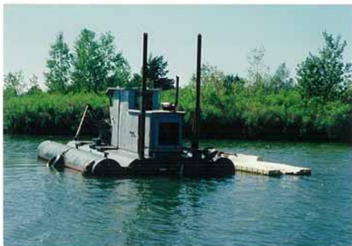
Figure 3-13: Hydraulic dredge for maintenance of North Pond inlet channel.
